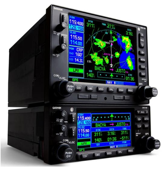
Garmin GNS 430W/530W. The first LPV capable GPS unit for general aviation. Over 130,000 made between 1998 and 2012.
