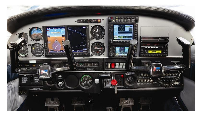
Piper PA28 with Garmin G600 EFIS and dual GNS-W.
