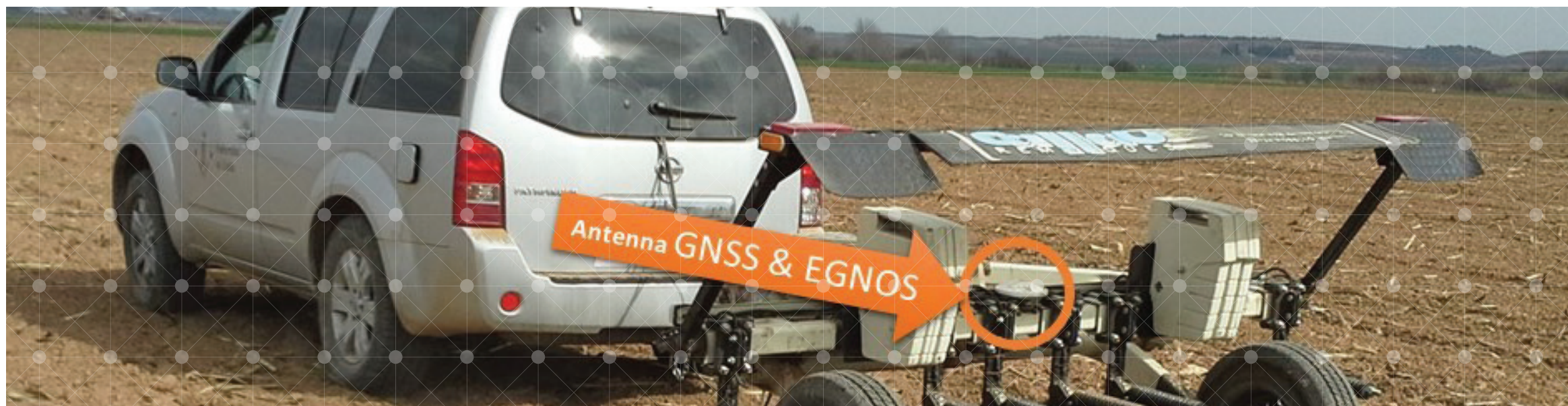
Figure 1. Veris 3100 Soil EC Surveyor of the University of Lleida with GNSS and EGNOS receiver
