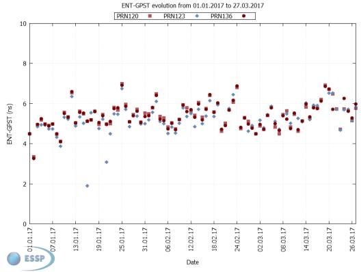
Figure 30 – ENT-GPS offset evolution<sup>10</sup>
