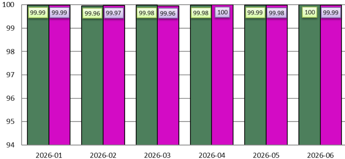
Figure 2 – Trend of EGNOS SIS Availability per GEO for the past 6 months (in green PRN 136; in purple PRN 121)
