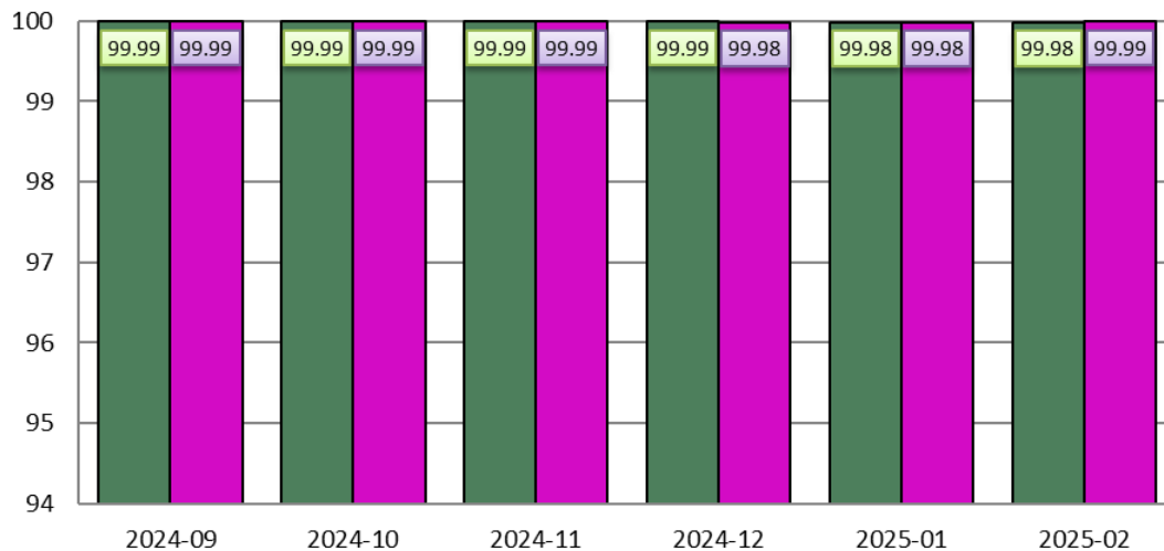
Figure 2 – Trend of EGNOS SIS Availability per GEO for the past 6 months (in green PRN 136; in purple PRN 123)
