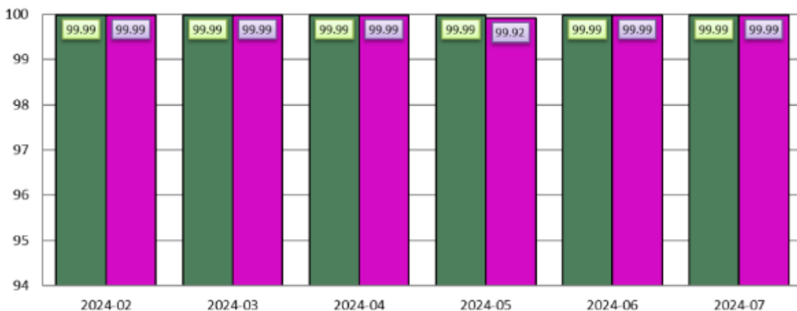
Figure 2 – Trend of EGNOS SIS Availability per GEO for the past 6 months (in green PRN 136; in purple PRN 123)
