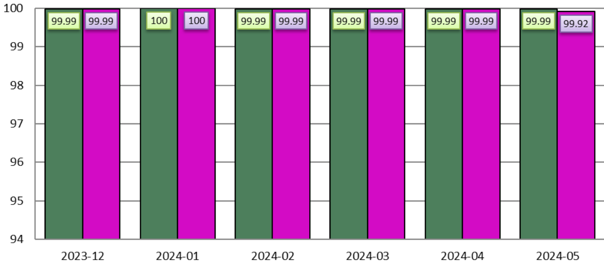
Figure 2 – Trend of EGNOS SIS Availability per GEO for the past 6 months (in green PRN 136; in purple PRN 123)
