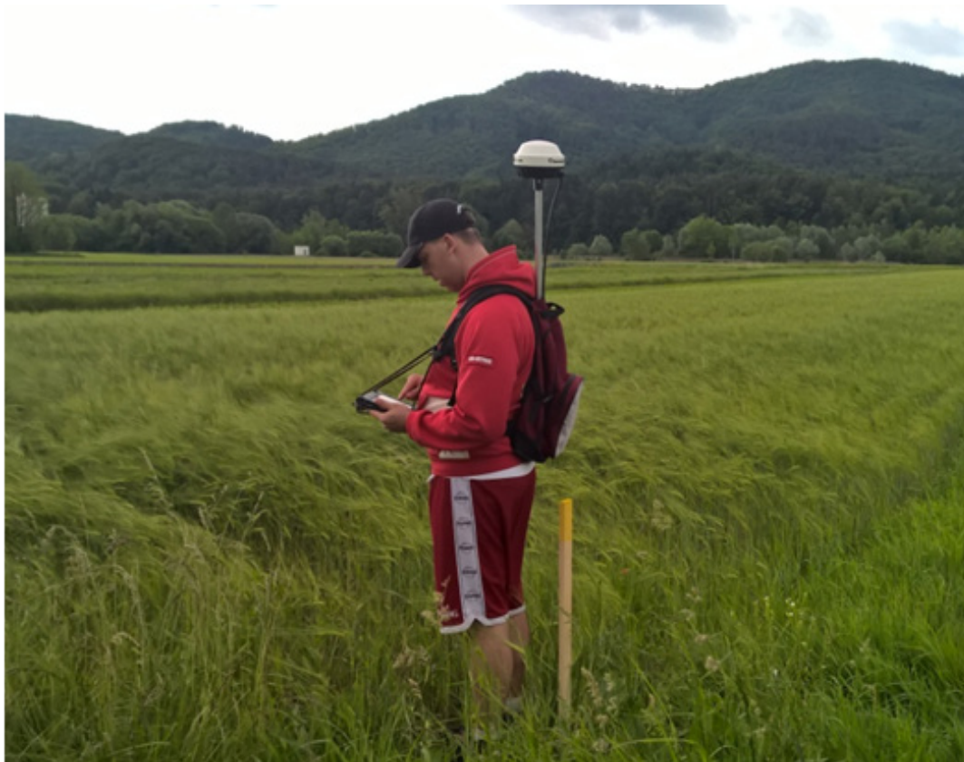
Field inspector from GZC performing an OTSC with portable GNSS equipment that uses EGNOS
