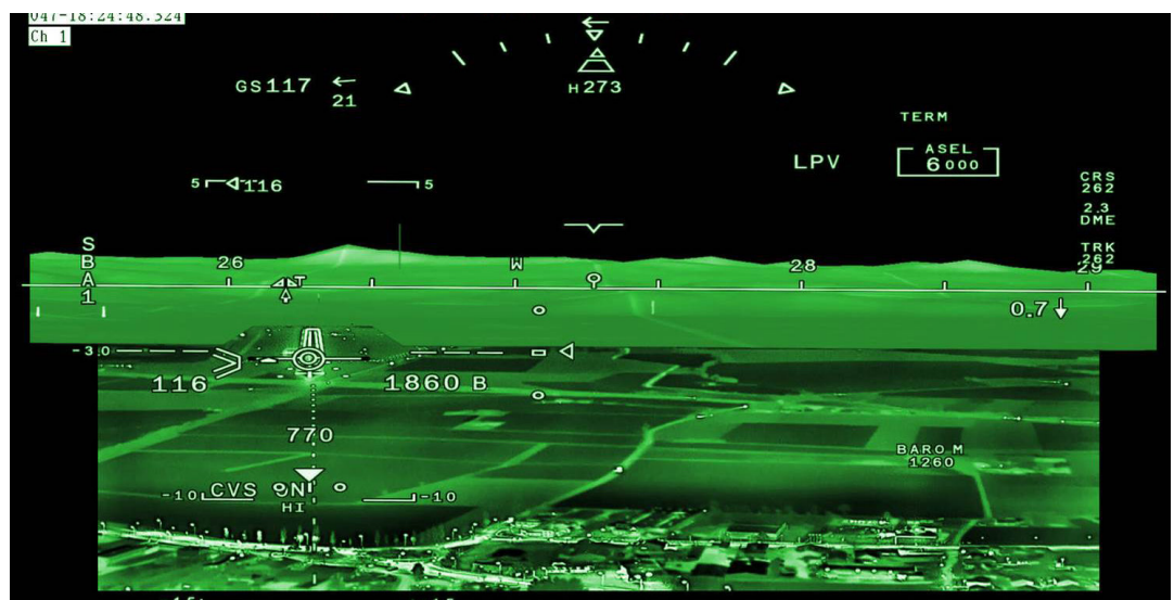
LPV approach with Enhanced Vision System from Dassault Aviation
