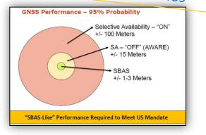
Towards curved segments with SBAS CS-ACNS Issue 2 – EGNOS used for geometric altitude for RNP-AR Enhanced and Synthetic vision systems minima below 200ft & reduction of RVR SBAS receivers (ETSO C145/146) present the maximum values of accuracy & availability
