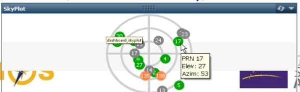
3. The SF-3050 receiver locates and tracks **SBAS** satellites at run-time, building a list of satellites that contribute to navigation solution.
