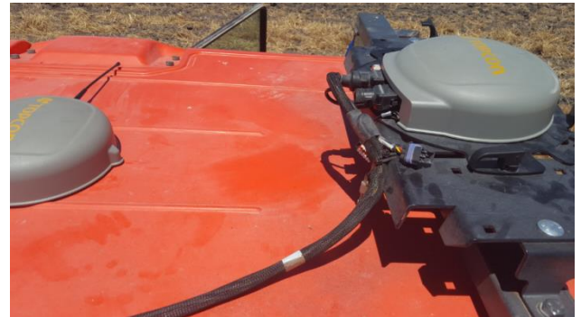
Figure 10: Topcon AGI-4 receivers used for the test (left: receiver fed by EDAS DGPS, right: receiver fed by Topcon's HiperV RTK base).
