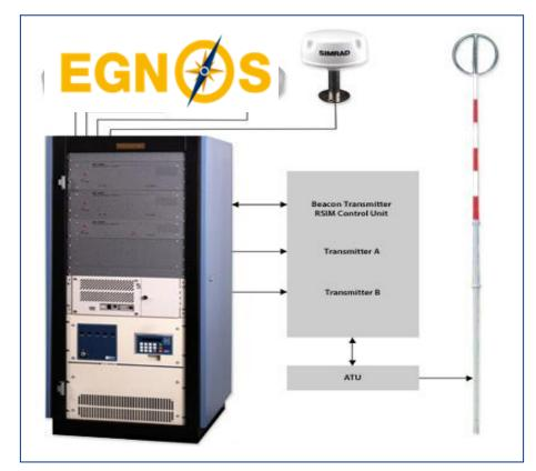
DGNSS station: GNSS receiver + MF transmitter. Courtesy: MxMarine
